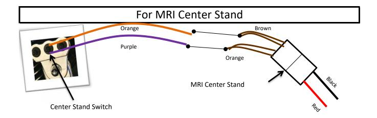
Tie both MRI Wires Together On Each Side Then Connect Them To My Purple & Orange Wires. Check Stand Operational Direction Before Soldering/Crimping Wires.
